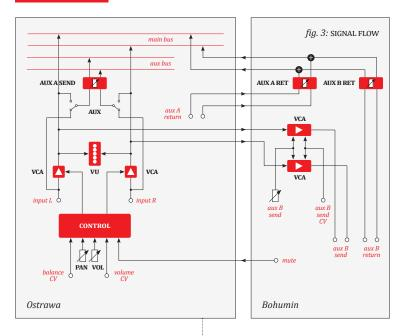
the amount of send can be controlled manually and via the additional VCAs inside Bohumin. The corresponding inputs accept bipolar voltages. A CV of 0 to +8V increases the amount of send relative to what is set with the knob, while negative CV of 0 to -8V gradually attenuates the signal even with AUX B SENDS LEVEL attenuators fully open.
