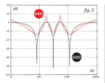
in a 2-notch and 3-notch frequency response, respectively, and can be used as a faux stereo pair to widen and spatially animate the signal. Of course, the outputs can also be used independently, as they each have a unique character.
