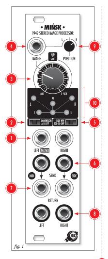
ed for the exact cancellation of components that are identical, but out of phase. What is sometimes surprising is that applying the same sum and difference to M and S reverts the whole process—which is precisely how we get back to left (L) and right (R) at the end.
