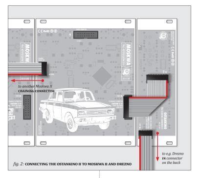
With the switch set to the BIT OUT position, each Ostankino II bit output (both on the panel and the Leibniz connector) sends a digital value (on/off) of the bit corresponding to the CV set for the currently active sequence step. Starting with the least significant bit at output 1 (bit 0) and ending with the most significant bit at output 8 (bit 7). The values present at the outputs change when the sequence is advanced to the next step to reflect
