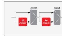
cells and is delivered to the output after 48 cycles of the clock. In other words, the data is digitally (and losslessly) delayed.
