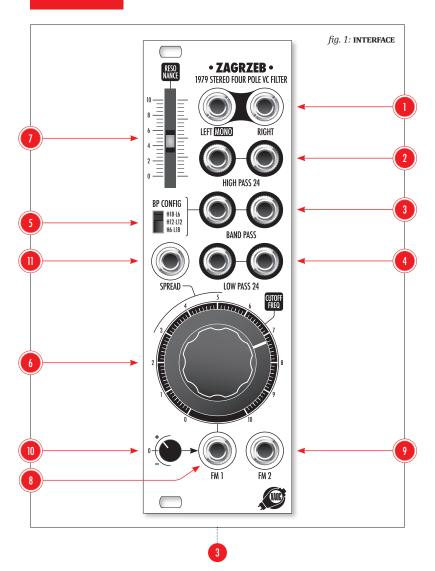
diate combinations are different variants of band pass (an asymmetric +6/-18dB, a symmetric +12/-12dB, and another asymmetric +18/-6dB) covering a wide spectrum between dark, mellow, boxy, honky, and harsh—and all that in stereo!
