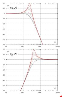
and H6 L18. Different slopes result in less or more radical filtering of components below and above the center cutoff frequency yielding significantly diverse timbres. Please note that the middle symmetric response features two 12dB/ oct slopes that are twice as steep (hence more selective) as a classic 2-pole SVF.
